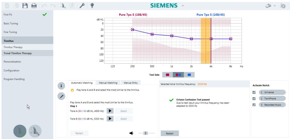
Figure 7. Tonal Tinnitus Therapy screen in Connexx 8.2 showing a Manually Entered pitch match as 3333 Hz, with the Frequency Check completed and the notch activated in all three listening programs.
