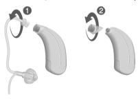
Screw on the new adapter and tube.
